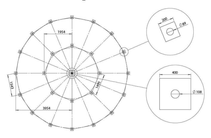
It is possible to use a band or monolithic foundation; combining of perimeter piles and concrete support in the center; other types of foundations.
